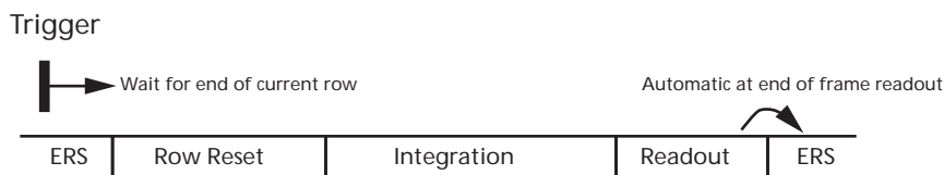
Figure 33: Entering and Leaving a Global Reset Sequence
