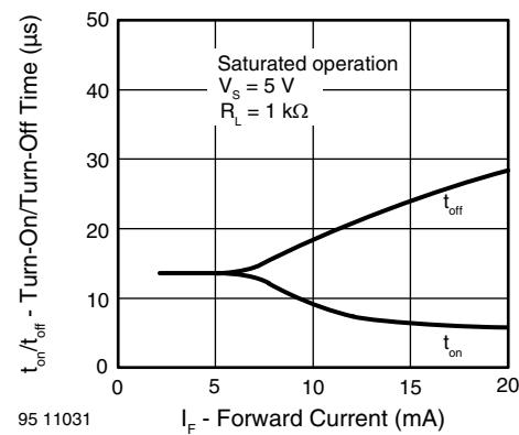
Fig. 18 - Turn-On/Turn-Off Time vs. Forward Current
