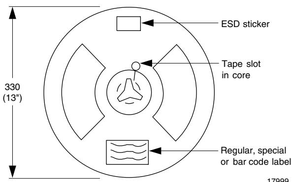
Fig. 20 - Reel Dimensions (3000 units per reel)
