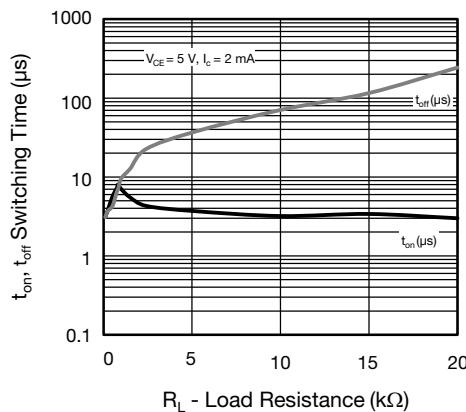
Fig. 16 - Switching Time vs. Load Resistance
