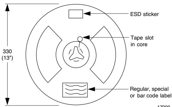
Fig. 20 - Reel Dimensions (3000 units per reel)
