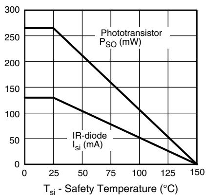
Fig. 4 - Derating Diagram
