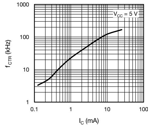
Fig. 15 - Cut-off Frequency (-3 dB) vs. Collector Current
