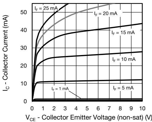
Fig. 7 - Collector Current vs. Collector Emitter Voltage (non-saturated)
