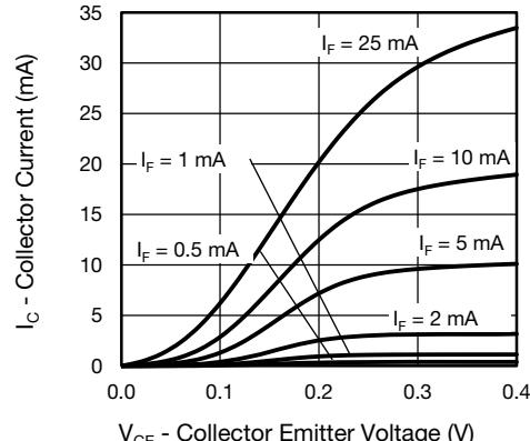
Fig. 9 - Collector Current vs. Collector Emitter Voltage (saturated)
