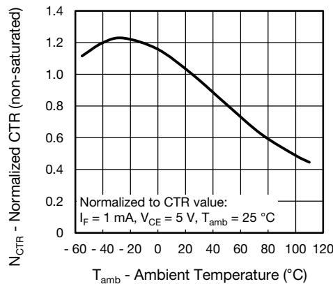
Fig. 11 - Normalized Current Transfer Ratio vs.
