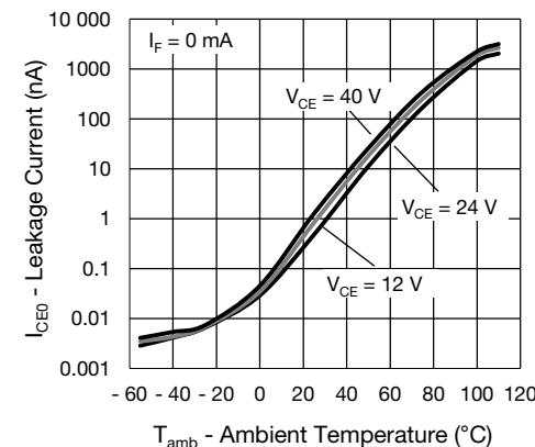
Fig. 8 - Collector Emitter Current vs. Ambient Temperature
