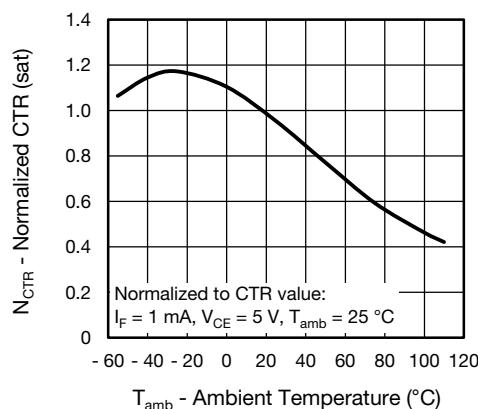
Fig. 10 - Normalized Current Transfer Ratio vs.
