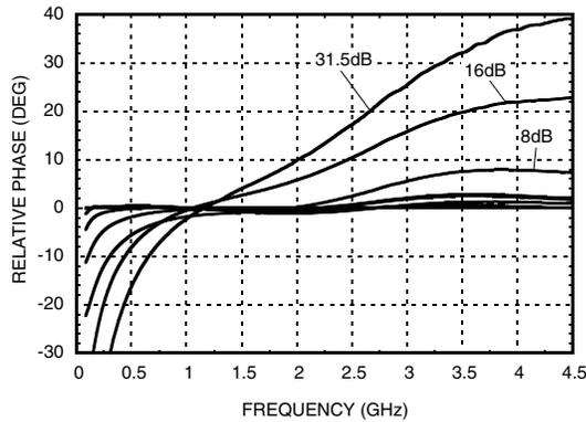
**Step Attenuation vs. Attenuation State**
