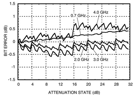
**0.5 dB LSB GaAs MMIC 6-BIT DIGITAL VARIABLE GAIN AMPLIFIER, 0.5 - 4 GHz**
