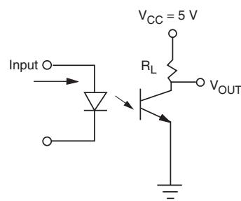
Fig. 3 - Test Circuit
