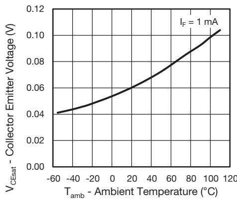
Fig. 9 - Collector Emitter Voltage vs. Ambient Temperature
