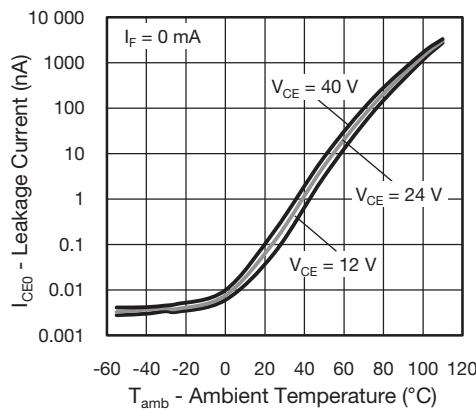
Fig. 7 - Collector Emitter Current vs. Ambient Temperature
