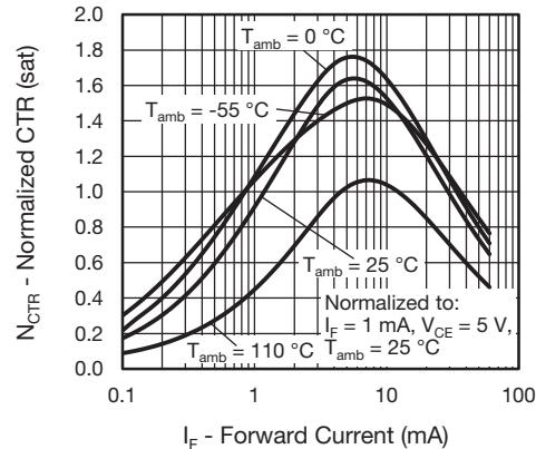
Fig. 12 - Current Transfer Ratio vs. Forward Current (saturated)
