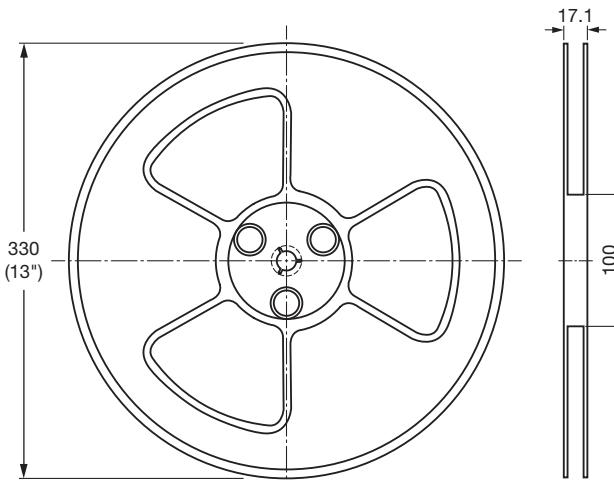
Fig. 18 - Reel Dimensions (3000 units per reel)
