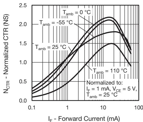
Fig. 13 - Current Transfer Ratio vs. Forward Current (non-saturated)
