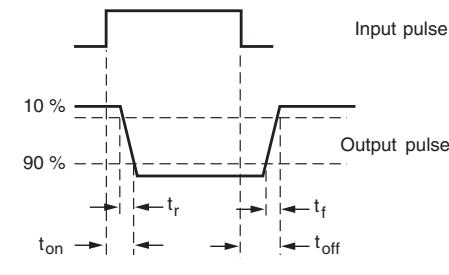
Fig. 4 - Test Circuit and Waveforms
