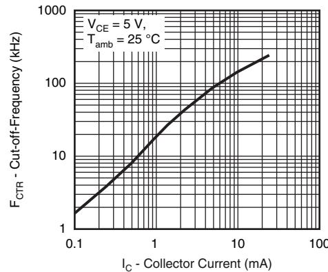
Fig. 14 - Cut-off Frequency (- 3 dB) vs. Collector Current
