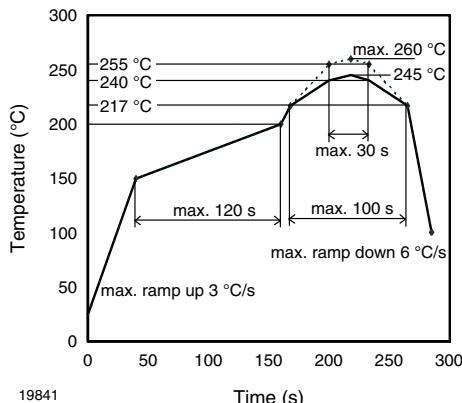
Fig. 20 - Lead (Pb)-free Reflow Solder Profile
