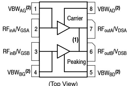
Figure 1. Pin Connections
