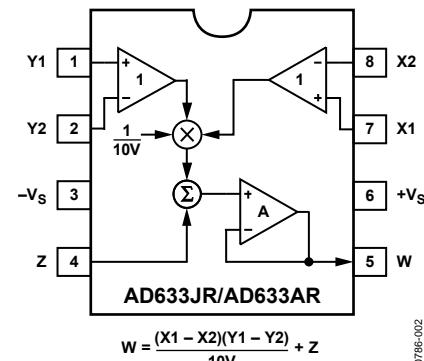
Figure 3. 8-Lead SOIC
