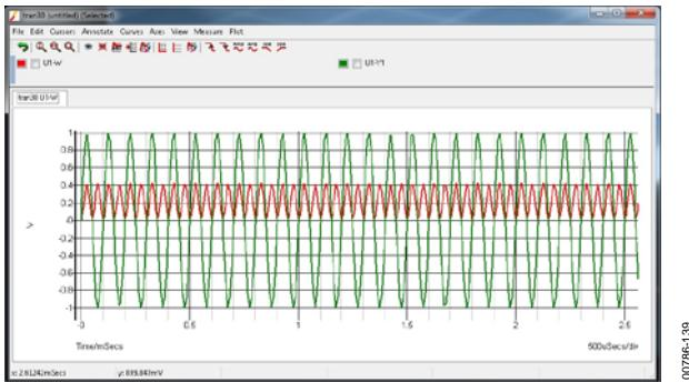
*Figure 39. Frequency Doubler Response Graph Displayed in SiMetrix*
