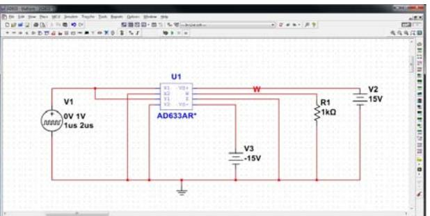
Figure 28. Pulse Circuit Schematic Created in Multisim
