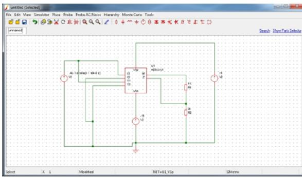
*Figure 38. Frequency Doubler Circuit Schematic Created in SiMetrix*
