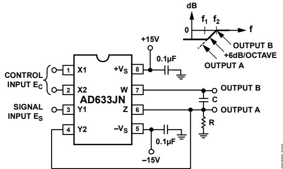
Figure 21. Voltage-Controlled, High-Pass Filter
