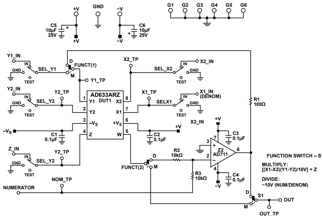
Figure 49. Schematic of the AD633 Evaluation Board
