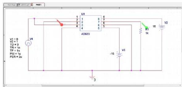
Figure 34. Pulse Circuit Schematic Created in PSPICE
