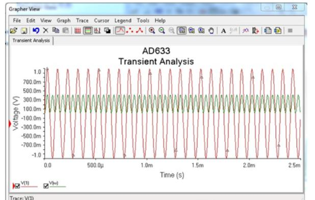
Figure 27. Frequency Doubler Response Graph Displayed in Multisim
