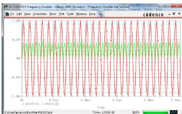
Figure 33. Frequency Doubler Response Graph Displayed in PSPICE
