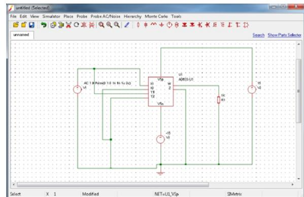
*Figure 40. Pulse Circuit Schematic Created in SIMetrix*
