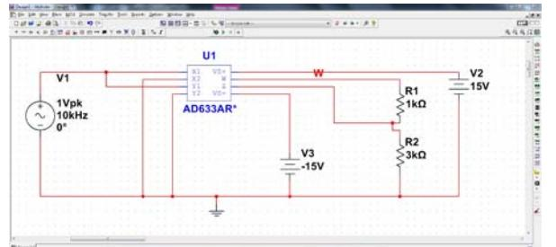
Figure 26. Frequency Doubler Circuit Schematic Created in Multisim
