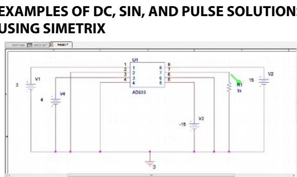
Figure 36. Simple Circuit Schematic Created in SIMetrix
