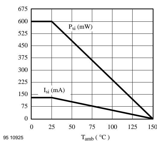
Figure 4. Derating diagram
