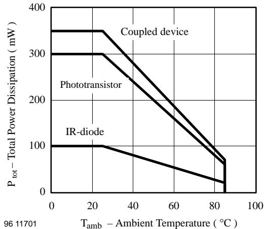
Figure 6. Total Power Dissipation vs.
