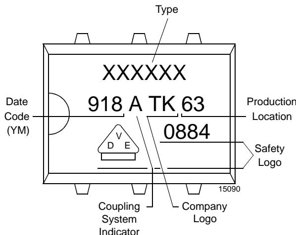
Figure 12. Marking example
