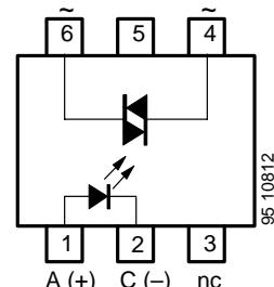
Note: Pin 5 must not be connected
