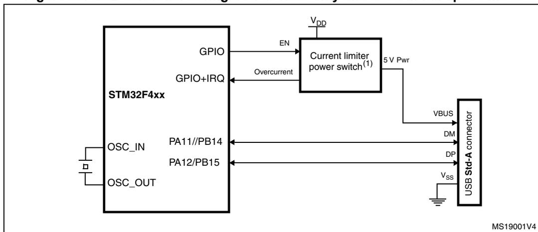
1. The current limiter is required only if the application has to support a  $V_{BUS}$  powered device. A basic power switch can be used if 5 V are available on the application board.
