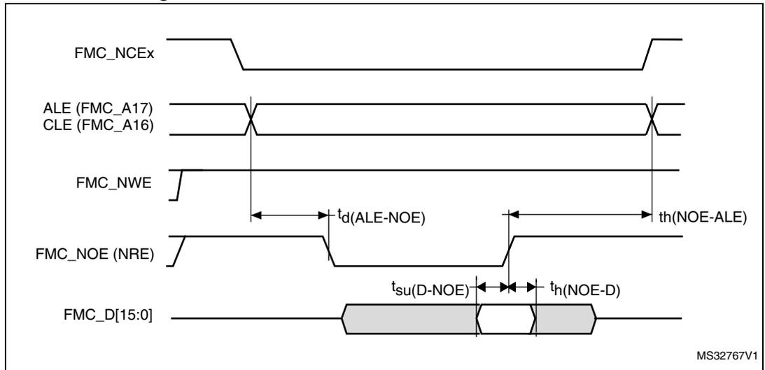
Figure 59. NAND controller waveforms for write access
