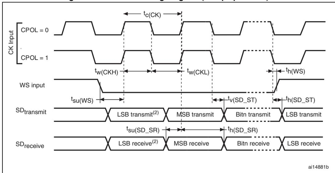
1. LSB transmit/receive of the previously transmitted byte. No LSB transmit/receive is sent before the first byte.
