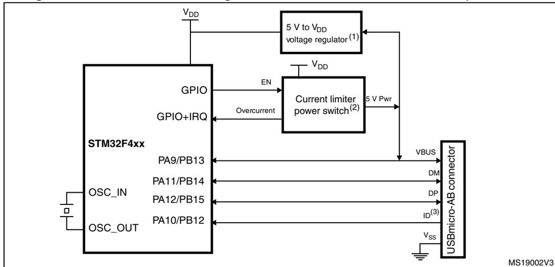
1. External voltage regulator only needed when building a V<sub>BUS</sub> powered device.
