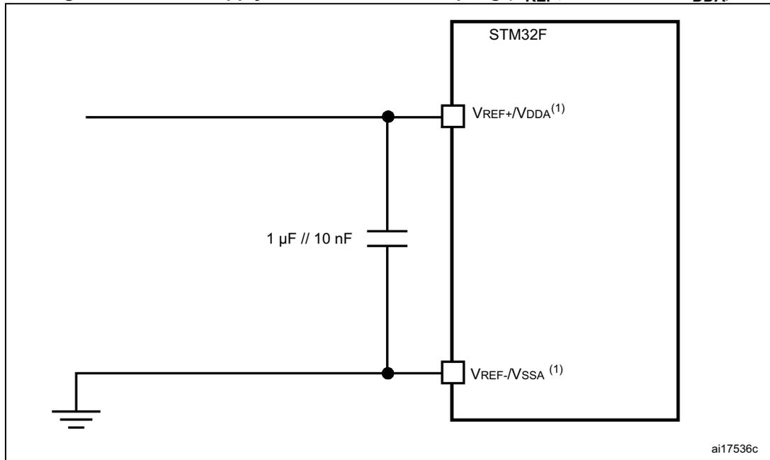
1.  $V_{REF+}$  and  $V_{REF-}$  inputs are both available on UFBGA144.  $V_{REF+}$  is also available on LQFP100, LQFP144, and WLCSP81. When  $V_{REF+}$  and  $V_{REF-}$  are not available, they are internally connected to  $V_{DDA}$  and  $V_{SSA}$ .
