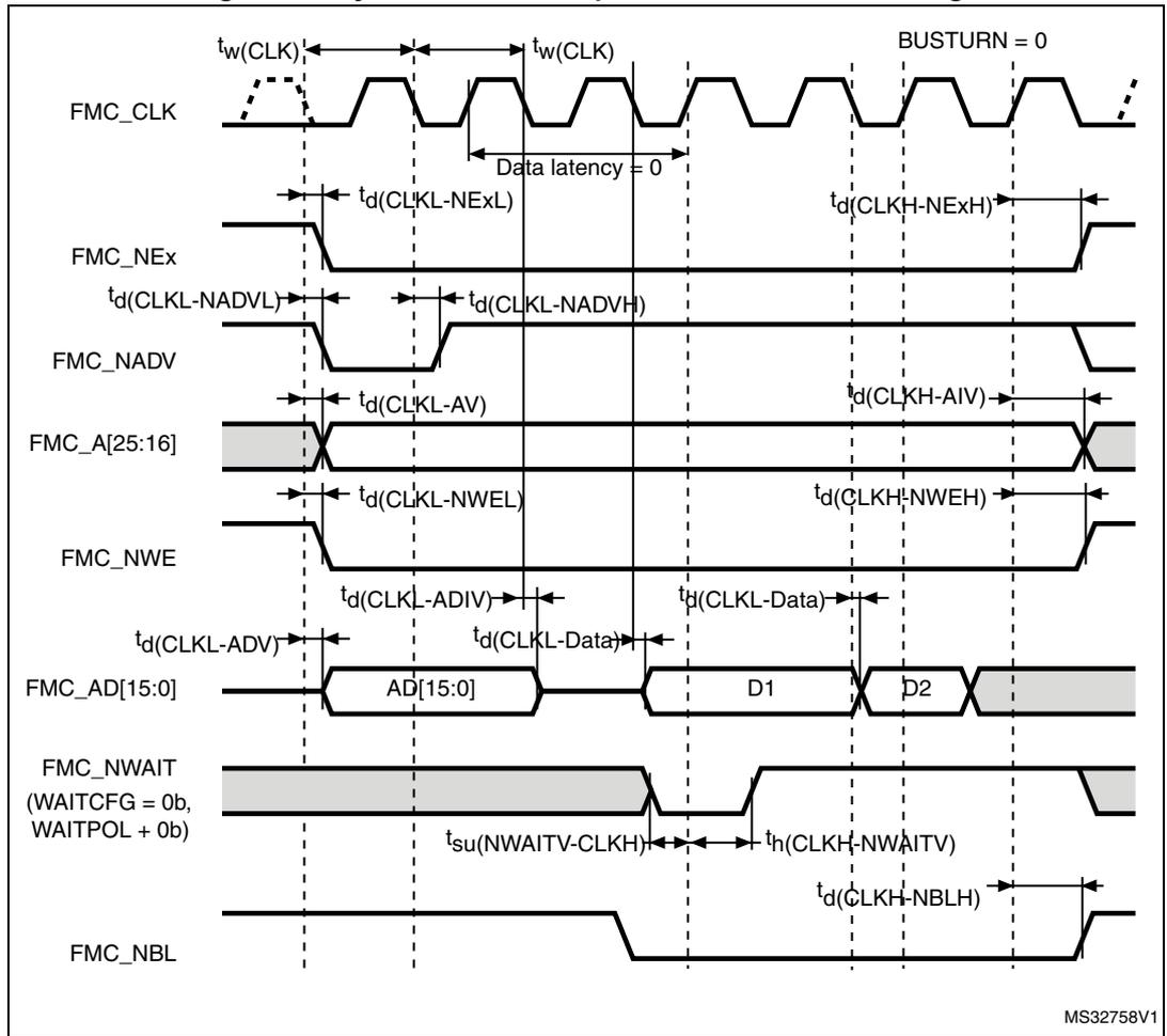
Table 95. Synchronous multiplexed PSRAM write timings<sup>(1)(2)</sup>
