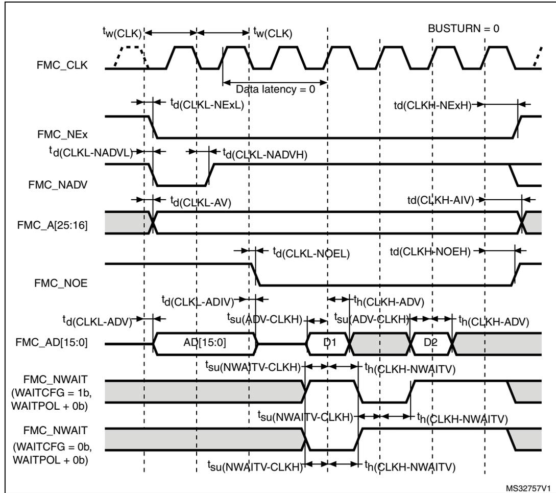
Table 94. Synchronous multiplexed NOR/PSRAM read timings<sup>(1)(2)</sup>
