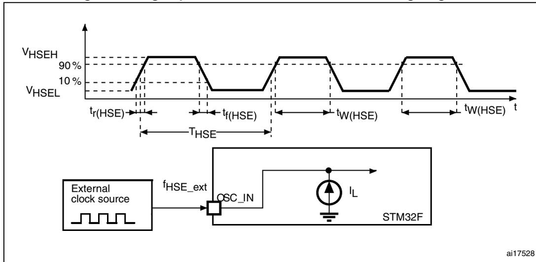
Figure 24. Low-speed external clock source AC timing diagram
