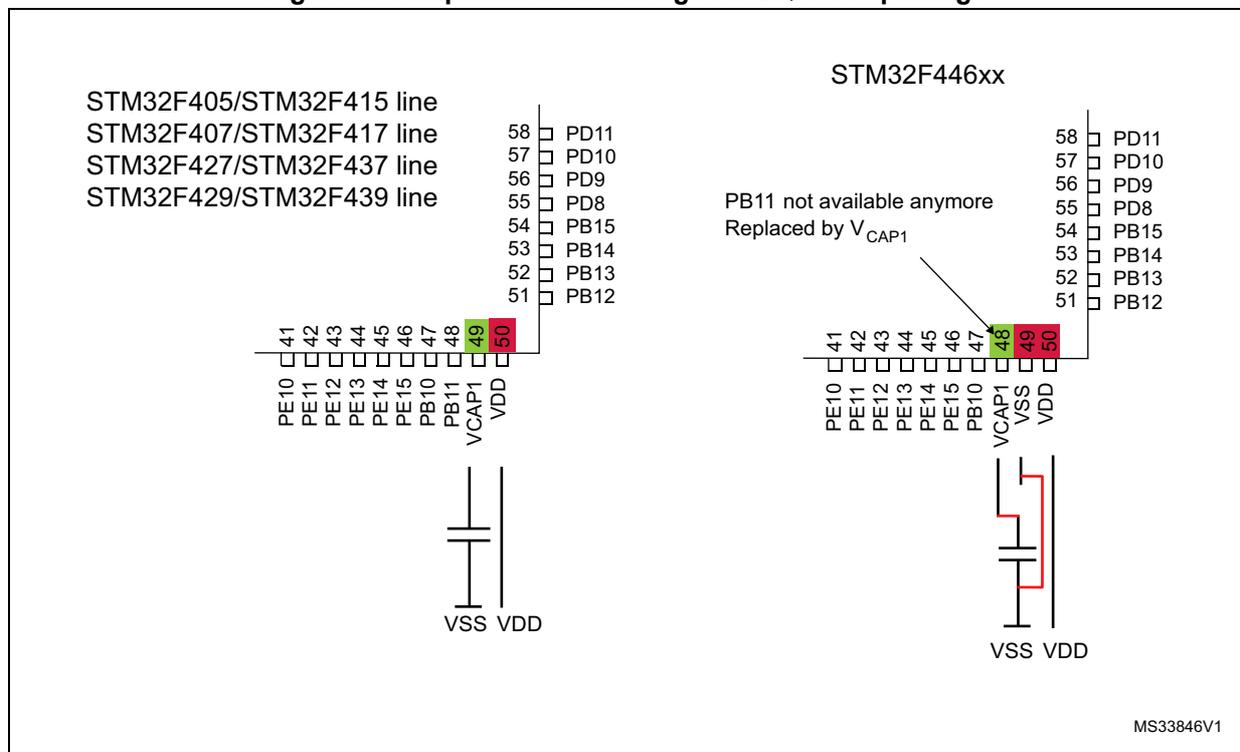
Figure 2. Compatible board for LQFP64 package
