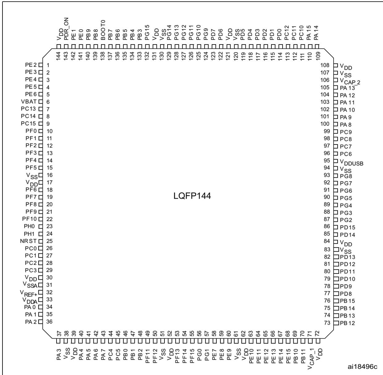
1. The above figure shows the package top view.
