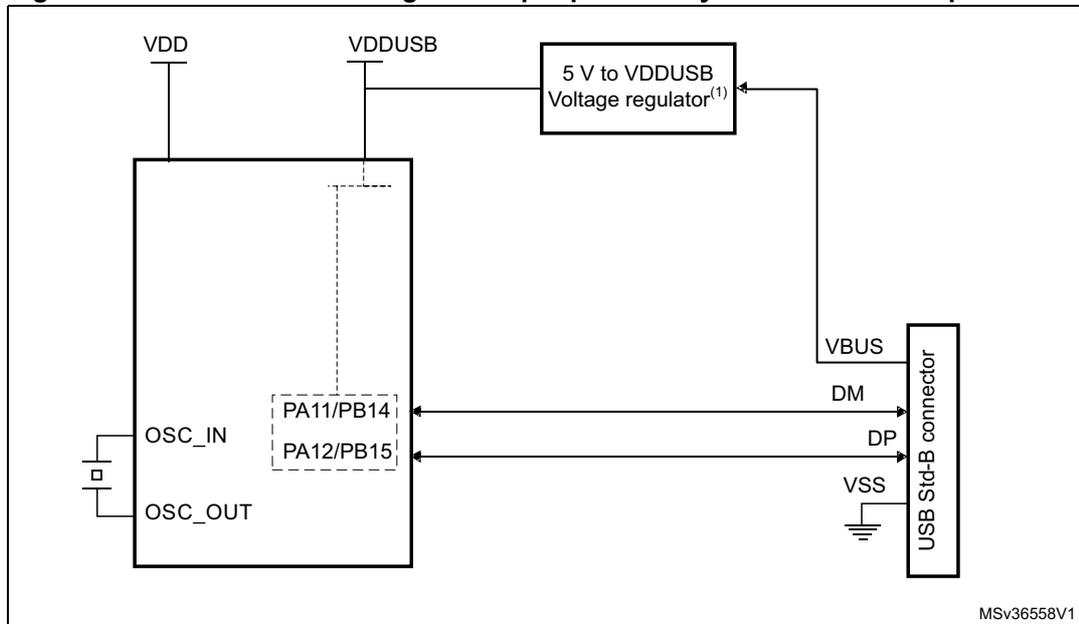
1. External voltage regulator only needed when building a  $V_{BUS}$  powered device.
