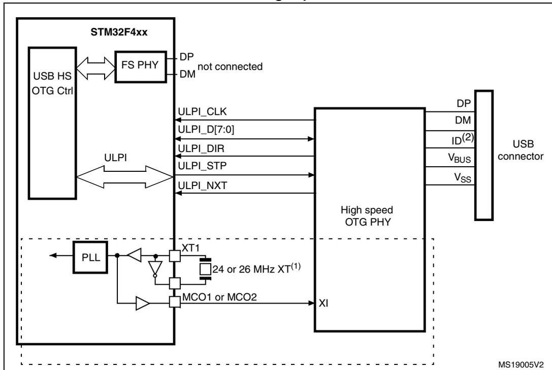
1. It is possible to use MCO1 or MCO2 to save a crystal. It is however not mandatory to clock the STM32F446xx with a 24 or 26 MHz crystal when using USB HS. The above figure only shows an example of a possible connection.
