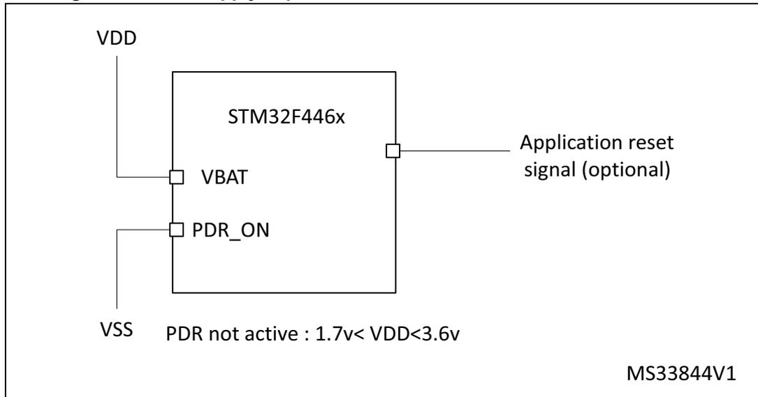
The  $V_{DD}$  specified threshold, below which the device must be maintained under reset, is 1.7 V.
