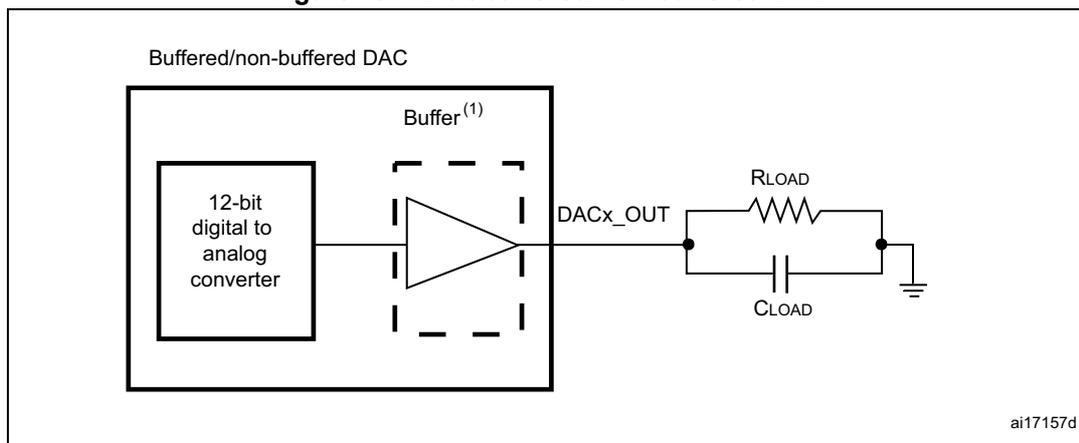
1. The DAC integrates an output buffer that can be used to reduce the output impedance and to drive external loads directly without the use of an external operational amplifier. The buffer can be bypassed by configuring the BOFFx bit in the DAC\_CR register.
