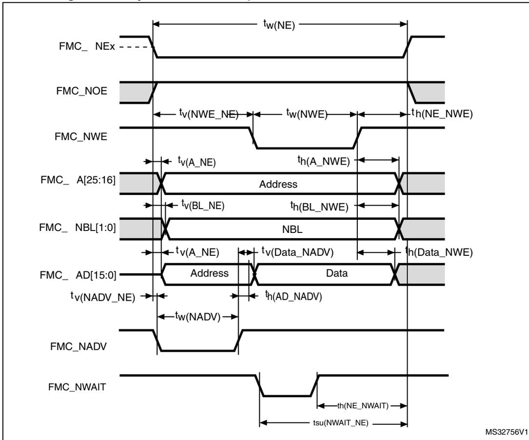
**Table 92. Asynchronous multiplexed PSRAM/NOR write timings<sup>(1)(2)</sup>**
