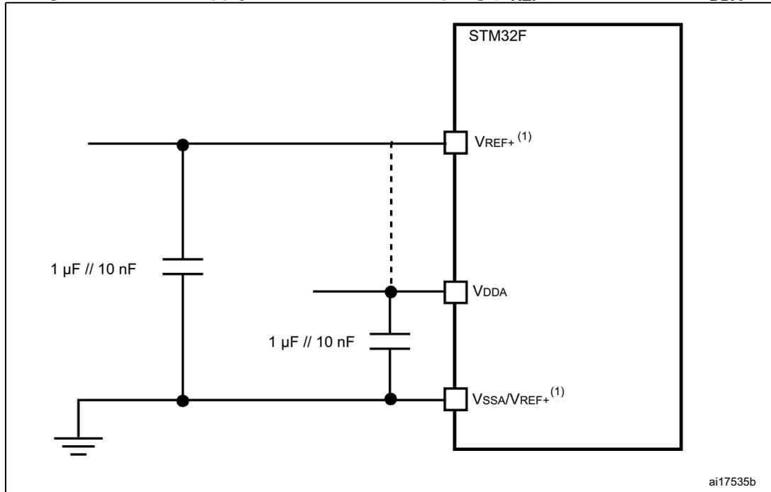
1.  $V_{REF+}$  and  $V_{REF-}$  inputs are both available on UFBGA144.  $V_{REF+}$  is also available on LQFP100, LQFP144, and WLCSP81. When  $V_{REF+}$  and  $V_{REF-}$  are not available, they are internally connected to  $V_{DDA}$  and  $V_{SSA}$ .
