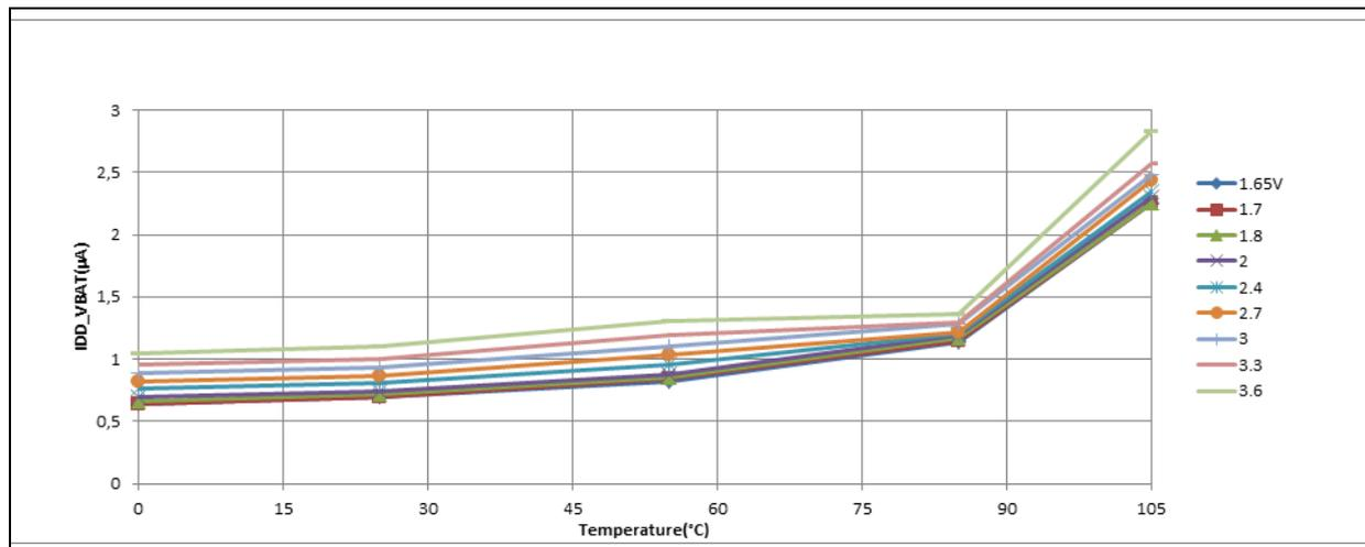
**Figure 22. Typical  $V_{BAT}$  current consumption (RTC ON/backup RAM OFF and LSE in high drive mode)**
