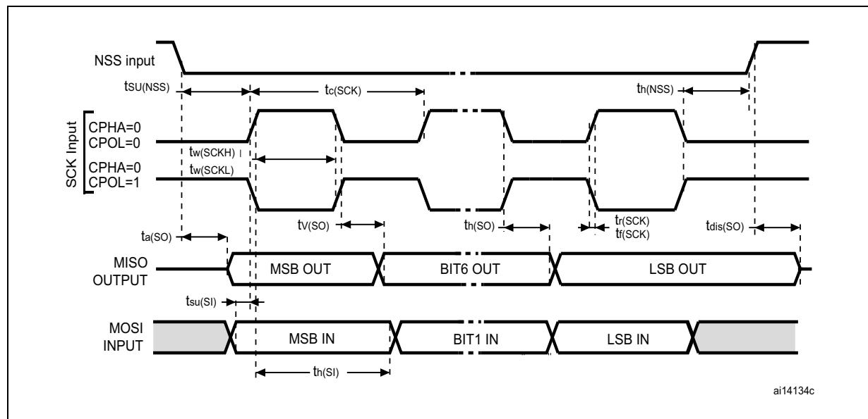
Figure 37. SPI timing diagram - slave mode and CPHA = 1
