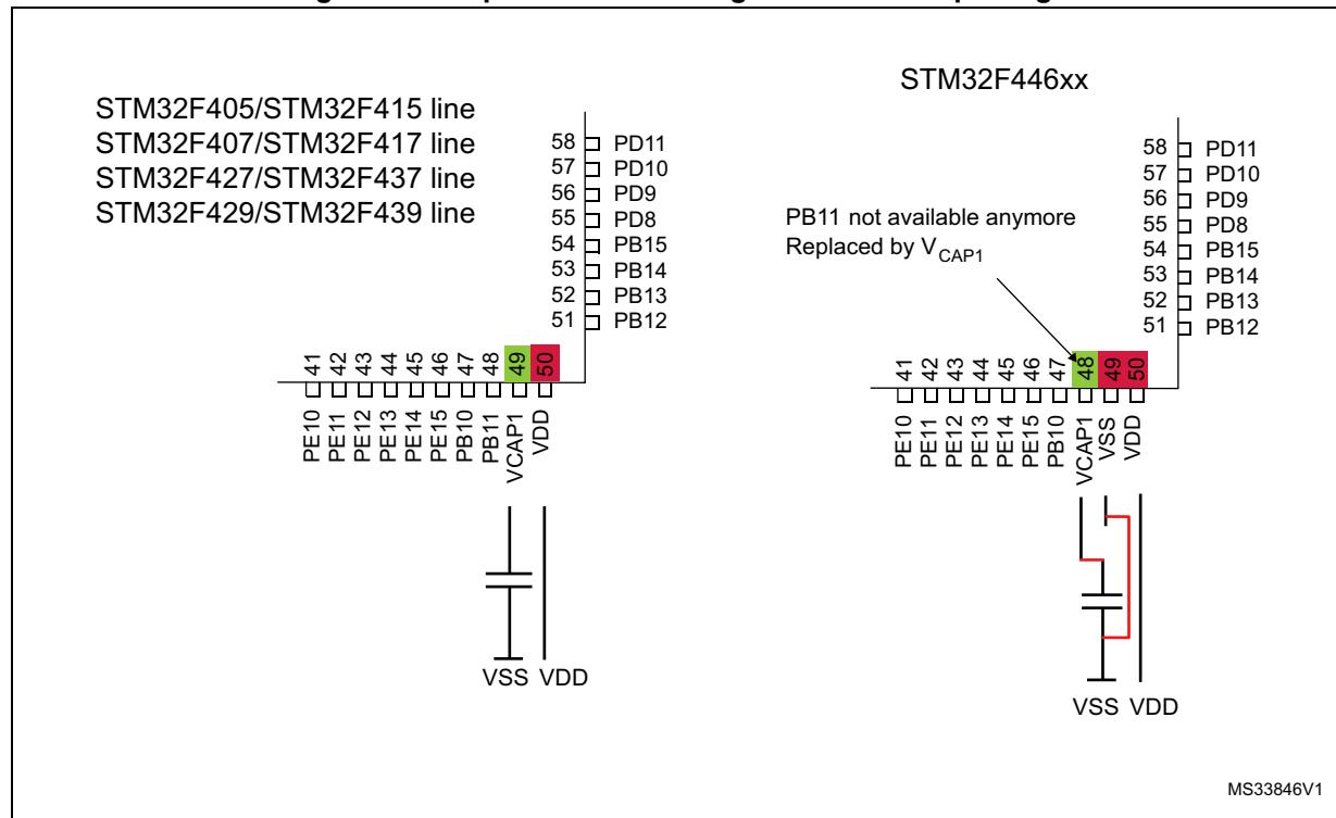
**Figure 2. Compatible board for LQFP64 package**
