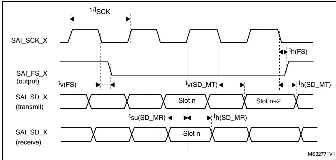
**Figure 42. SAI slave timing waveforms**
