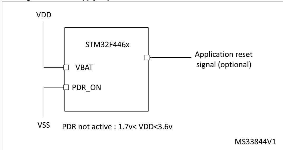
The  $\text{V}_{\text{DD}}$  specified threshold, below which the device must be maintained under reset, is 1.7 V.
