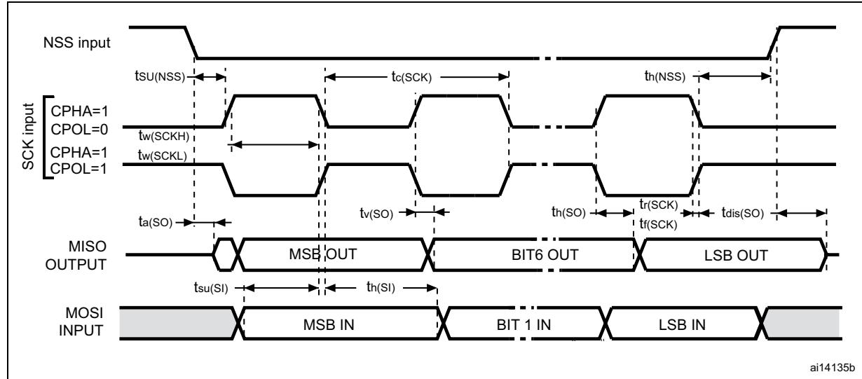
Figure 38. SPI timing diagram - master mode
