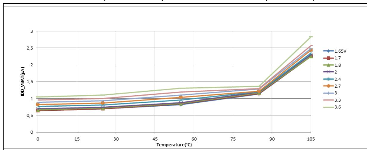
**Figure 22. Typical  $V_{BAT}$  current consumption
