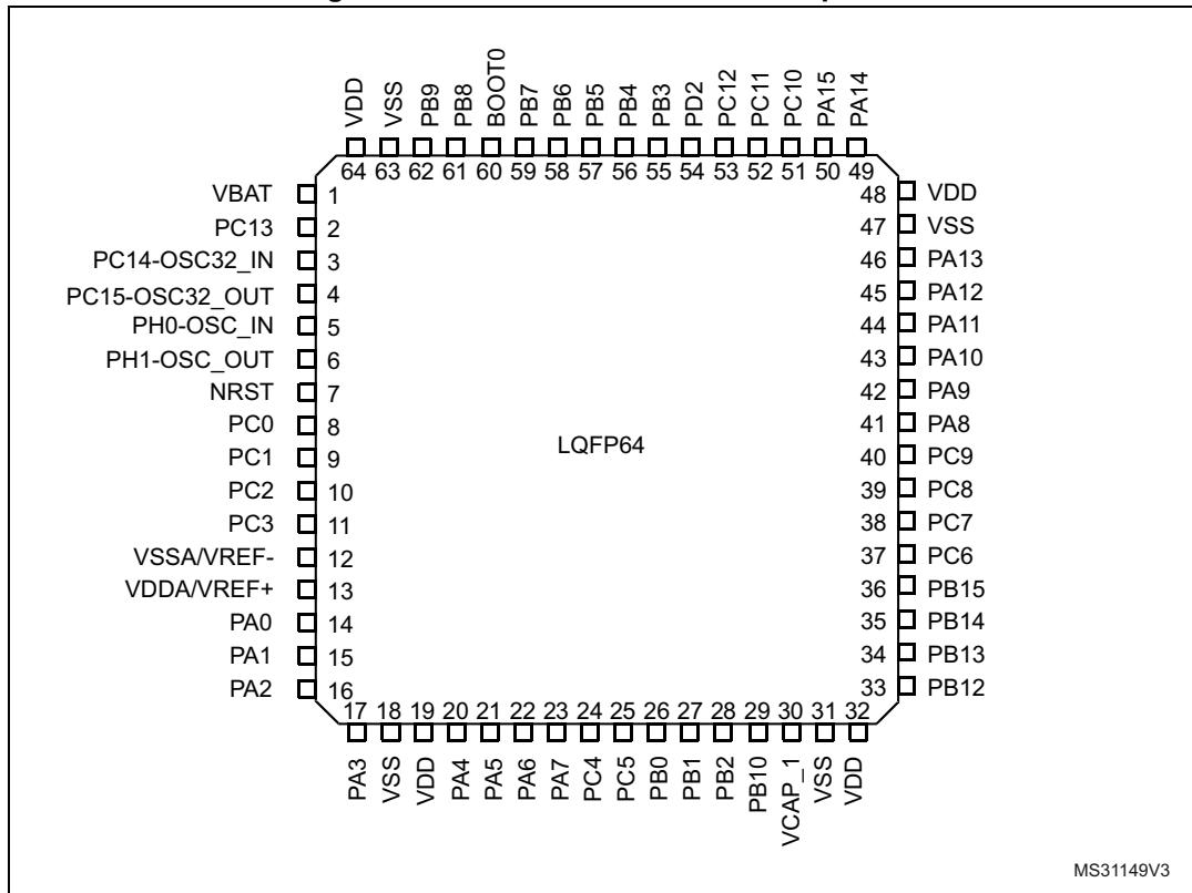
1. The above figure shows the package top view.
