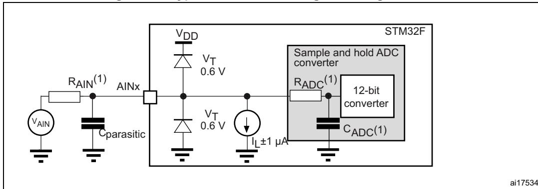
1. Refer to [Table 74](#) for the values of  $R_{AIN}$ ,  $R_{ADC}$  and  $C_{ADC}$ .
