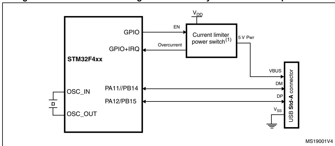
1. The current limiter is required only if the application has to support a  $V_{BUS}$  powered device. A basic power switch can be used if 5 V are available on the application board.
