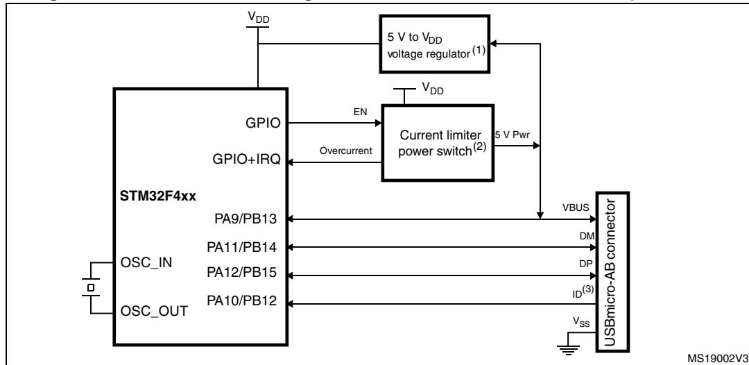
1. External voltage regulator only needed when building a  $V_{BUS}$  powered device.
