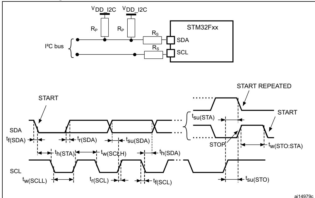
1. R<sub>S</sub> = series protection resistor.
