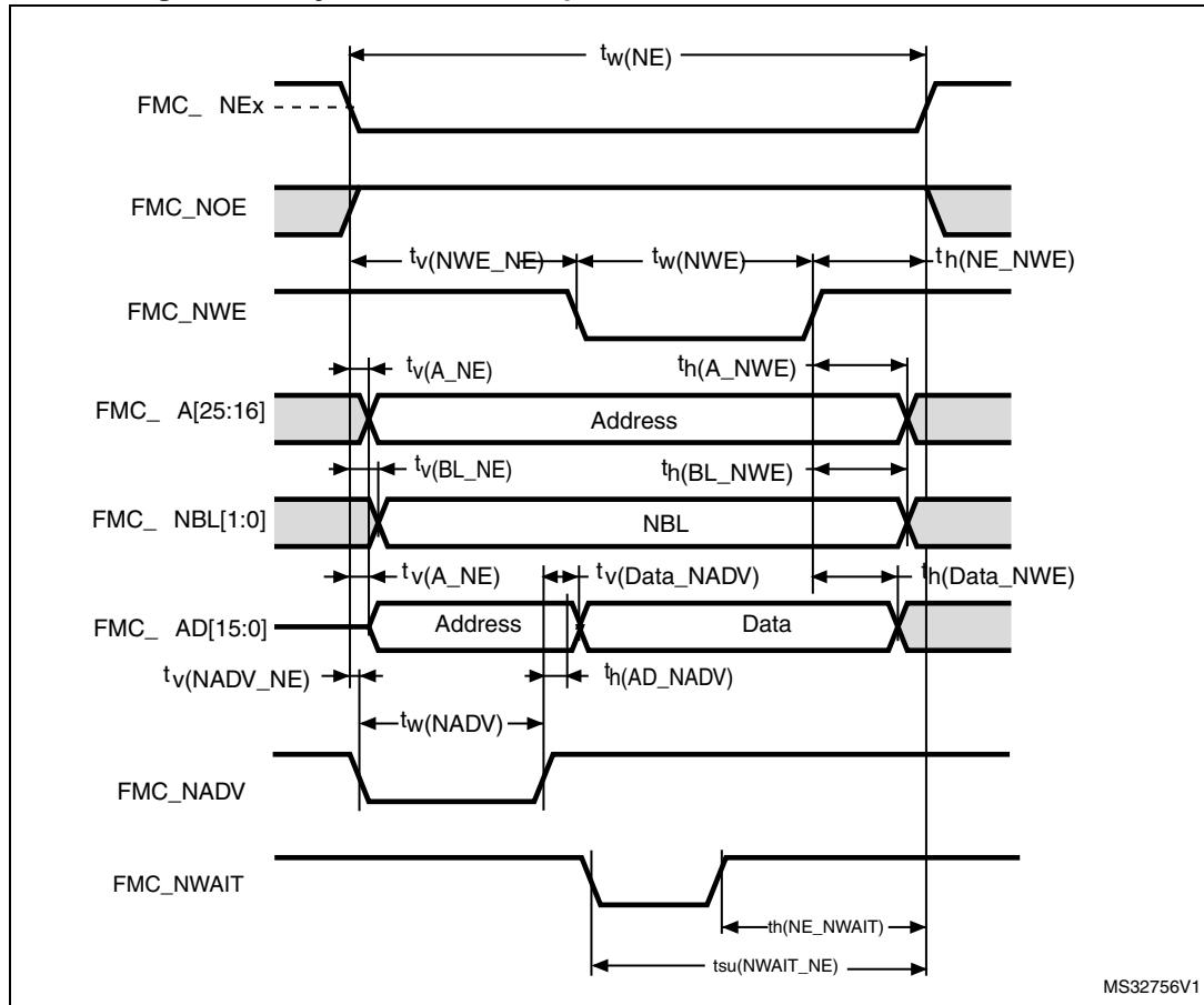
**Table 92. Asynchronous multiplexed PSRAM/NOR write timings<sup>(1)(2)</sup>**
