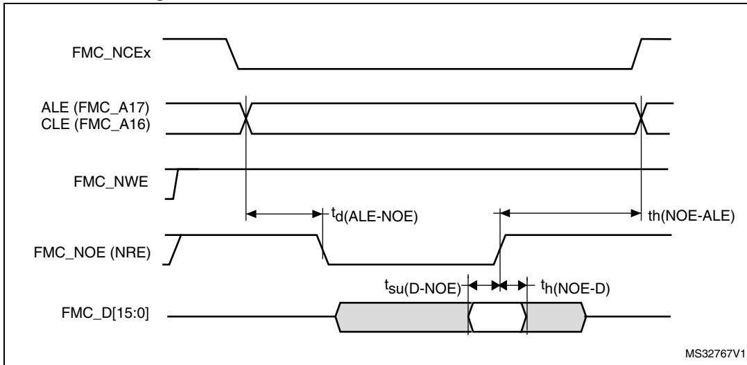
**Figure 59. NAND controller waveforms for write access**
