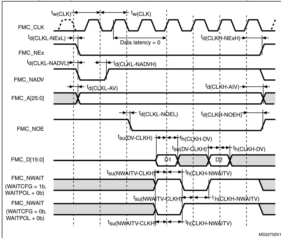
Table 96. Synchronous non-multiplexed NOR/PSRAM read timings<sup>(1)(2)</sup>
