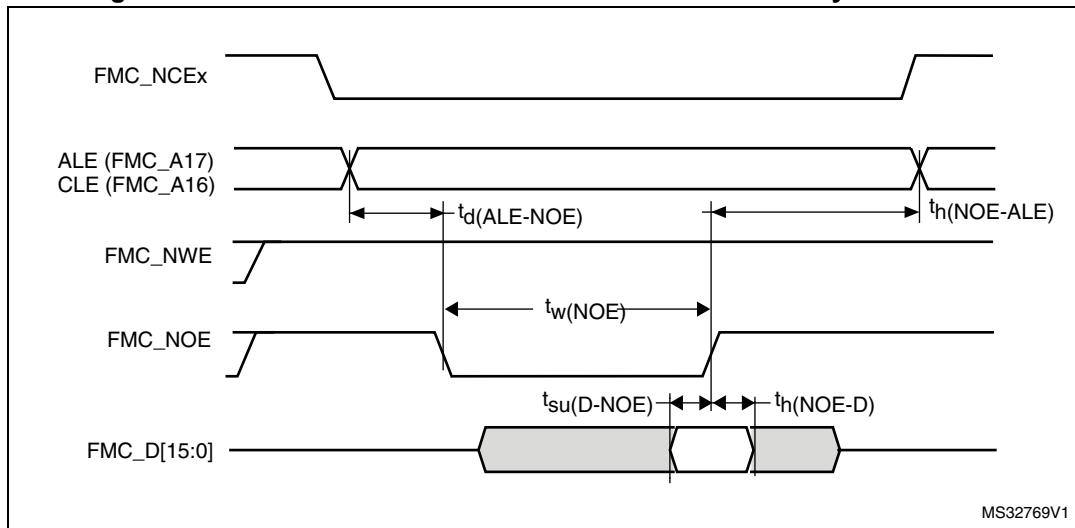
**Figure 61. NAND controller waveforms for common memory write access**
