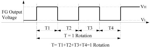
T = T1 + T2 + T3 + T4 = 1 Rotation  $T = \frac{60}{\text{rpm}}$
