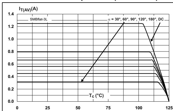
**Figure 4. Average and DC on-state current versus ambient temperature**
