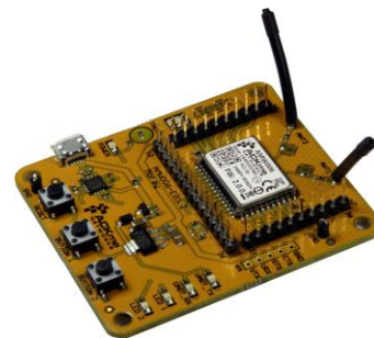
Figure 9 - AMW006-E03 eval board with wire antennas
