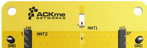
Figure 10 – Chip antenna layout example
