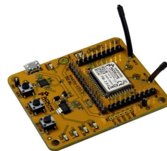
Figure 9 - AMW006-E03 eval board with wire antennas
