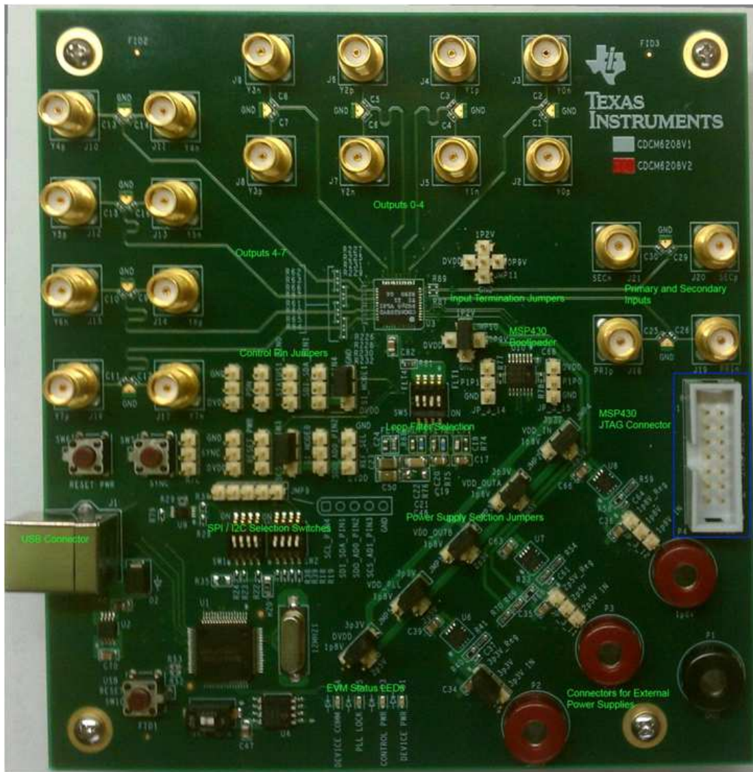
Figure 1. CDCM6208 Evaluation Board
