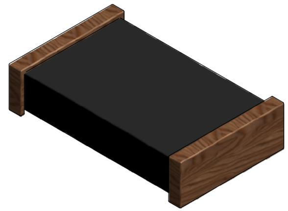
*Purchased Assembly Includes Walnut Sides, Steel Or Aluminum Chassis, Rubber Feet, 4 Lock Washers And 4 Assembly Screws.*
