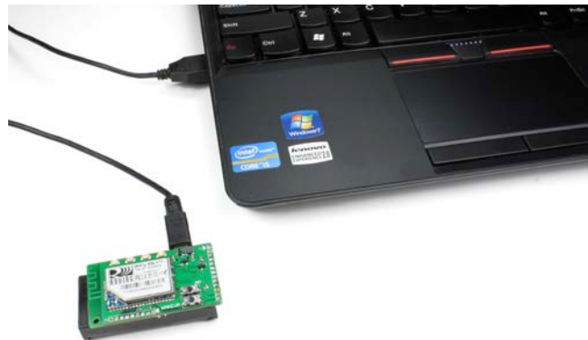
RN-171-EK Evaluation Board Hardware Setup
