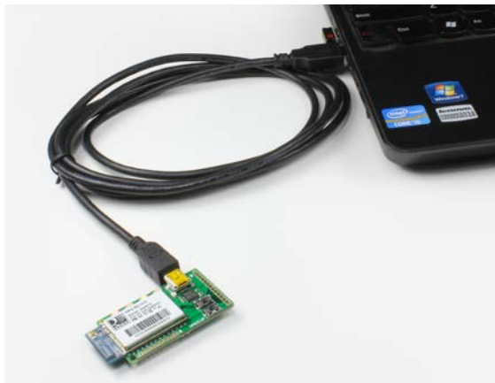
RN-131-EK Evaluation Board Hardware Setup
