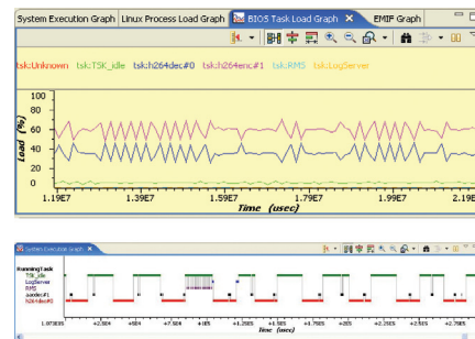
Screenshots from BIOS v6 Code Composer Studio, showing task CPU load and task priorities
