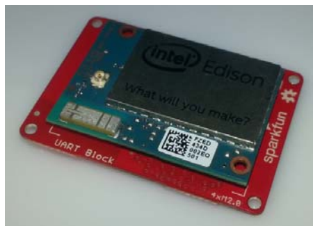
UART Block Installed
