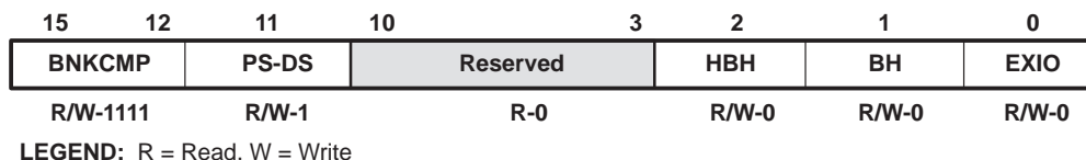
Figure 6. Bank-Switching Control Register (BSCR), MMR Address 0029h
