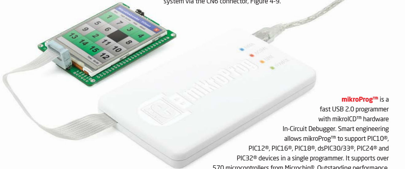
Figure 4-9: Connecting mikroProg™ to mikroMedia™
