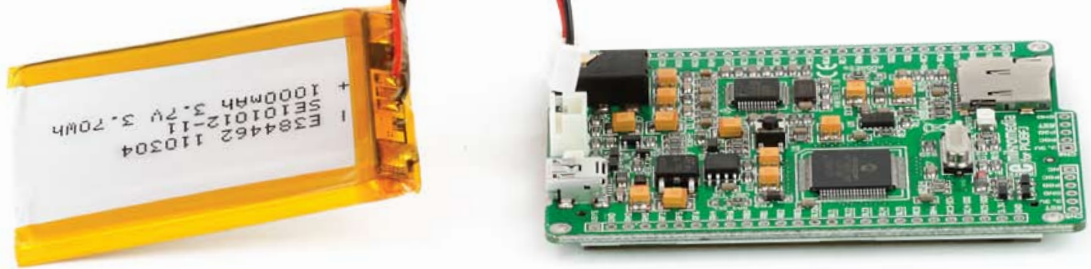
Figure 2-1: Connecting Li-polymer battery to mikromedia™ board
