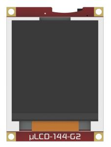
Embedded at the heart of the design is the **GOLDELOX** processor, which is driven by a highly optimised virtual core engine called **EVE** (Extensible Virtual Engine).
