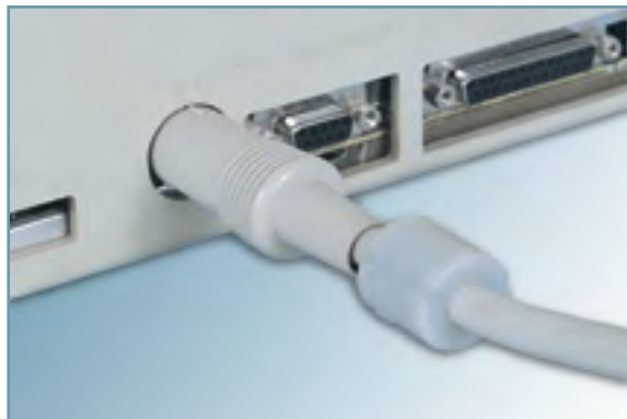
I/O cable with RFI suppressor.
