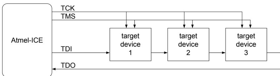
When connecting devices in a daisy-chain, the following points must be considered:
