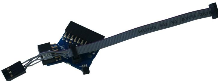
Figure 2-10. Atmel-ICE AVR Probe Connection
