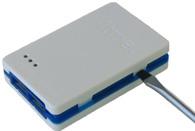
Figure 2-14. Opening the Atmel-ICE(3)
