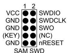
The Atmel-ICE is capable of streaming UART-format ITM trace to the host computer. Trace is captured on the TRACE/SWO pin of the 10-pin header (JTAG TDO pin). Data is buffered internally on the Atmel-ICE and is sent over the HID interface to the host computer. The maximum reliable data rate is about 3MB/s.
