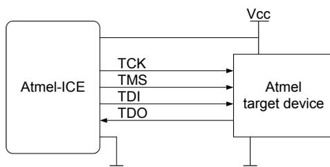
When designing an application PCB which includes an Atmel AVR with the JTAG interface, it is recommended to use the pinout as shown in [Figure 4-2, “AVR JTAG Header Pinout” on page 20](#). The Atmel-ICE can connect to both 100-mil and 50-mil variants of this pinout.
