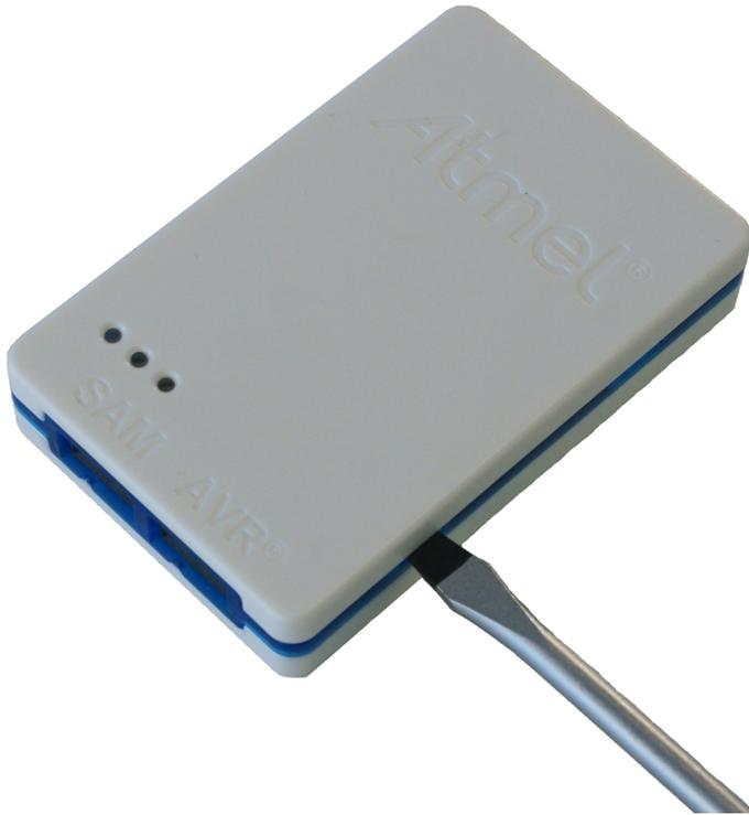
Figure 2-13. Opening the Atmel-ICE (2)
