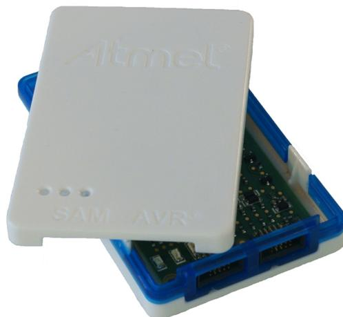
To close the unit again, simply align the top and bottom covers correctly, and press together firmly.
