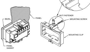
farthest forward slot possible. To achieve a proper seal, tighten the latch screws evenly until the unit is snug in the panel (Torque to approx. 28 to 36 in-oz [0.202 to 0.26 N-m]). Do not over-tighten the screws.
