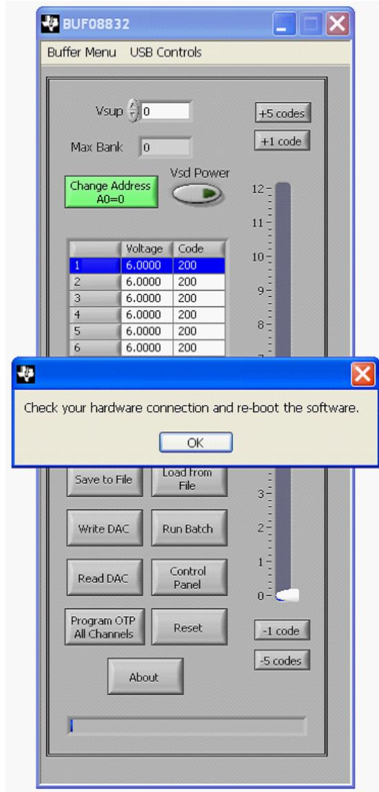
Figure 14. BUF08832EVM Software: No Communication with the USB\_DIG\_Platform
