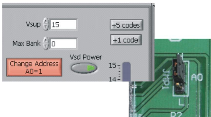
**Figure 15. BUF08832\_Test\_Board Jumper JMP1 Set For Logic '1'**
