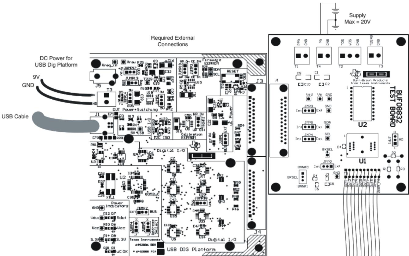
Figure 5. Typical Hardware Connections
