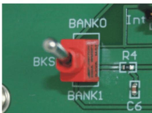
Figure 9. BKSEL Switch
