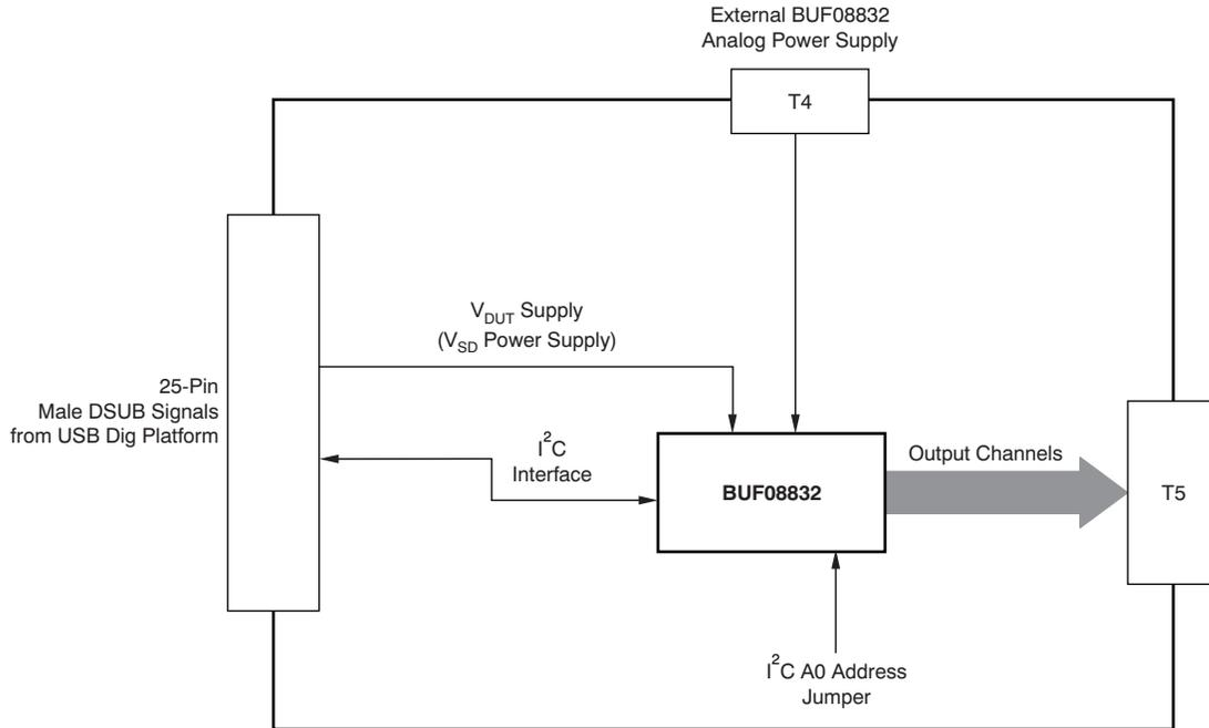
**Figure 3. BUF08832\_Test\_Board Block Diagram**
