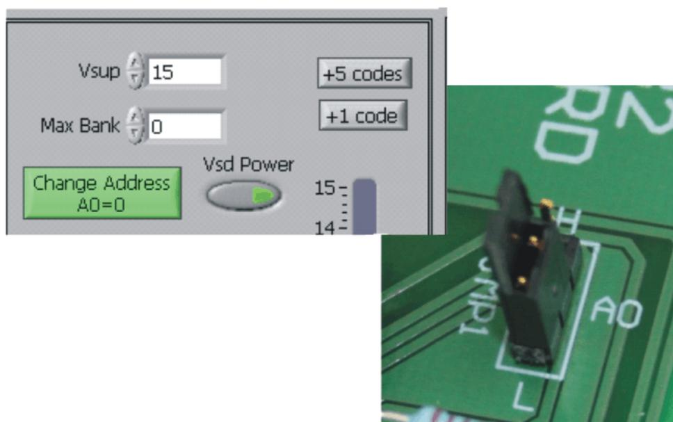
**Figure 16. BUF08832\_Test\_Board Jumper JMP1 Set For Logic '0'**
