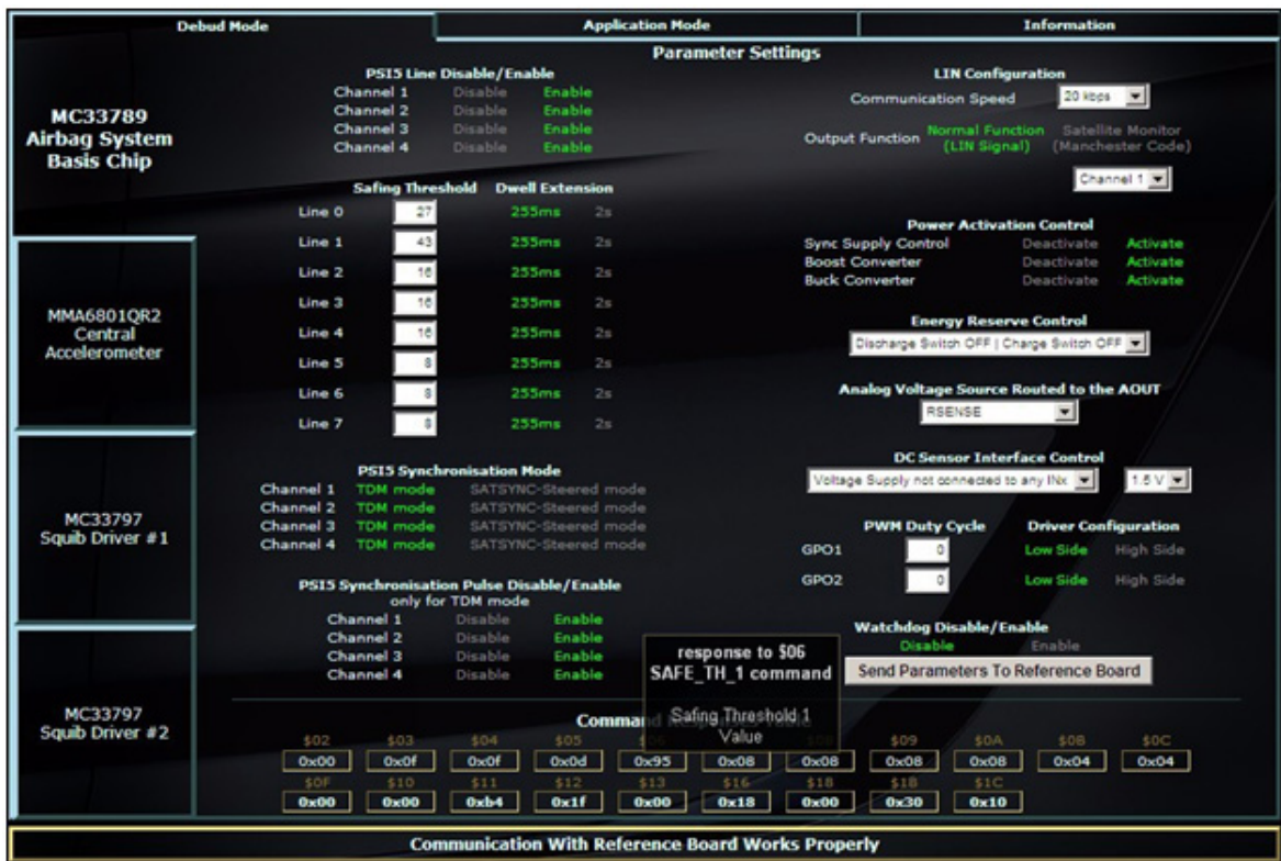
Figure 8. FreeMASTER Debug Page for the MC33789 Device
