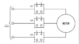
Three-phase motors may be controlled by solid-state relays as shown. A third SSR as shown is optional, but not necessary. The control windings may be connected in series or parallel. Care should be taken to ensure that the surge current drawn by the motor does not exceed the surge current rating of the SSR.
