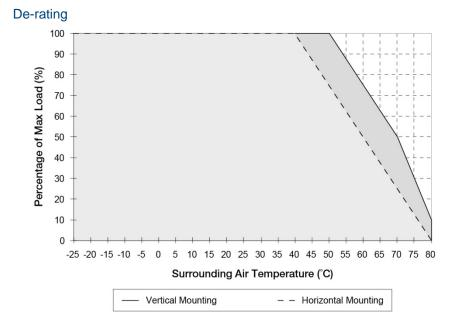
Fig. 1De-rating for Vertical Mounting Orientation<br/>> 50°C de-rate power by 2.5% / °C,<br/>> 70°C de-rate power by 4% / °C
