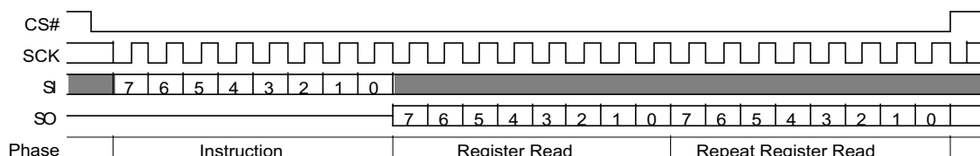
Figure 10.8 Read Bank Register (BRRD 16h) Command
