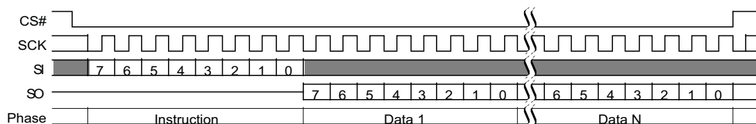
Figure 10.70 Password Read (PASSRD E7h) Command Sequence
