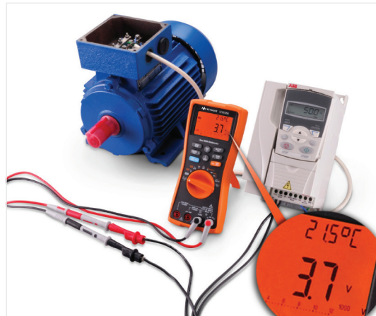
Figure 2. U1272A helps you identify the presence of stray voltage on a disconnected wire running parallel with the wire powering up the VFD to an industrial motor. The image on the right shows the U1272A in low impedance mode.
