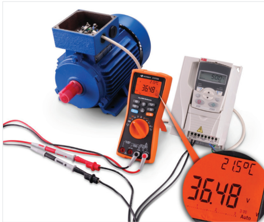
Figure 2. U1272A helps you identify the presence of stray voltage on a disconnected wire running parallel with the wire powering up the VFD to an industrial motor. The image on the right shows the U1272A in low impedance mode.
