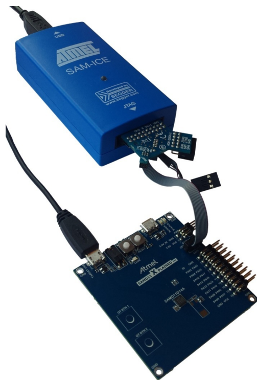
Figure 7-7. SAM-ICE using an Atmel-ICE Adapter
