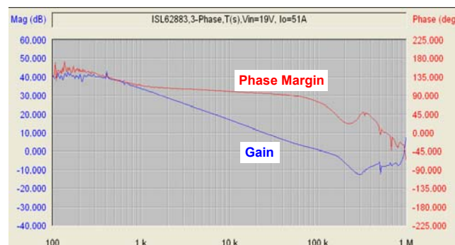
FIGURE 53. REFERENCE DESIGN LOOP GAIN T2(s) MEASUREMENT RESULT
