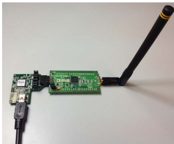
Figure 1 ADuCRF101 Mini Board and Emulator Board
