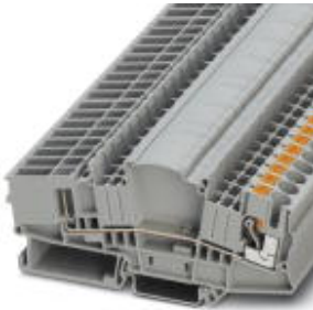
Feed-through terminal block, Connection method: Push-in connection, Cross section: 0.5 mm 2 -10 mm 2 , AWG: 20 - 10, Width: 8.2 mm, Color: gray
