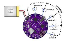
When you activate a switch, the trigger will be connected to ground, which is "low" or 0V. The software knows that when a trigger is low, it's time to play the proper audio file.
