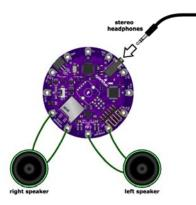
4. Connect a headphone to the headphone jack, **or** connect speakers to the left and right speaker terminals. (Note that when anything is plugged into the headphone jack, the speakers are disabled. This behavior can be changed if desired).
