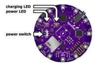
The board contains a **power switch** that is used to turn the board on and off. There are also two LEDs; a **red power LED** that will light up when the board is powered on, and a **yellow charge LED**. The charge LED will light up when the battery is being charged, and go out when it is full. (It is also
