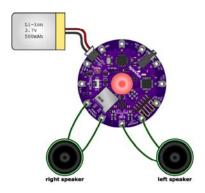
9. Turn the power switch ON. The red LED should light up, and after a few seconds, the rotary encoder will turn red, indicating the player is in "track" mode. (If the rotary encoder blinks, there was a startup problem, see the troubleshooting page for help.)
