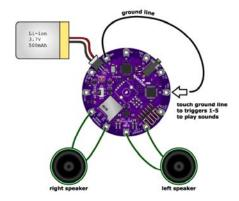
7. Wait a few seconds for the software to start up. Now, momentarily, connect the ground sew tap (marked GND) to one of the trigger terminals (marked T1 through T5). The audio file associated with that terminal should play through the speakers / headphone. If you don't hear anything, see the troubleshooting page.
