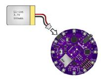
5. Plug a 3.7V single-cell Lipo battery into the JST connector. Note that a FTDI USB connection will not provide enough power to run the board, so a battery or other external power source is required.
