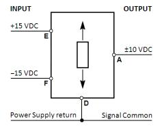
A through F: Connector pin assignments
