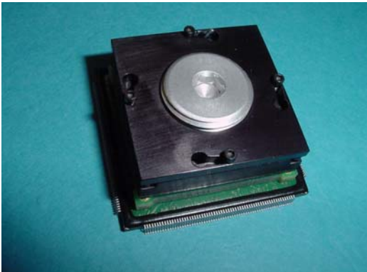
Figure 2. Assembled "CQFP to FBGA adapter socket" Adapter Board with socket (SI-SX32-ACQ256SFG484)
