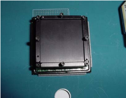
Figure 7. Assembly step 4 –place the compression plate on top of device
