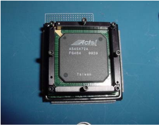
Figure 6. Assembly step 3 – place in FG484 in socket
