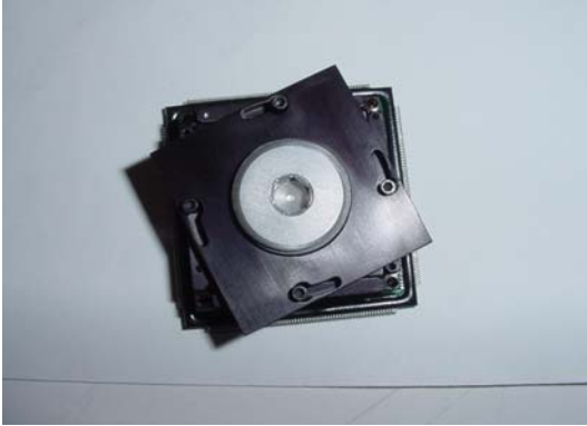
Figure 8. Assembly step 5 – put on top lid
