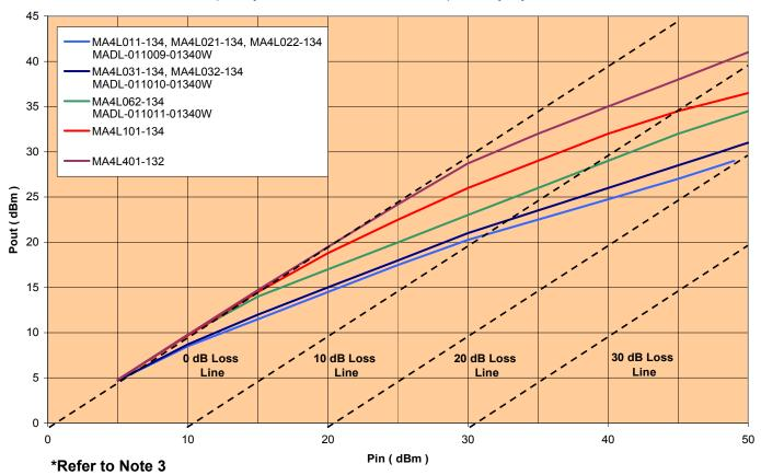
High Signal Performance: Measured in a single shunt diode (die) configuration attached directly to the gold plated RF ground of a  $50\Omega$ , SMA connectorized, test fixture using 2 mil thick conductive silver epoxy. Chip anode contact is thermo-compression wire bonded using a 1 mil. diameter gold wire onto a 7.2 mil thick Rogers 5880 Duroid microstrip trace. A shunt coil provides the D.C. return.
