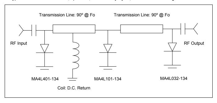
Typical +50dBm Peak Power, 1µS P.W., 0.001% Duty Cycle, +20dBm Flat Leakage Limiter Circuit
