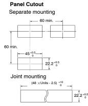
Waterproofing is not possible for joint mounting
