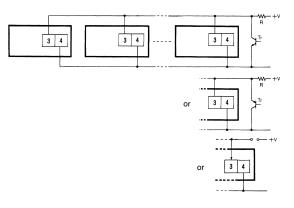
Note: H (Reset ON) level must be 4.5 V minimum.  $H = \frac{4.7 (k\Omega)/N + V}{2}$
