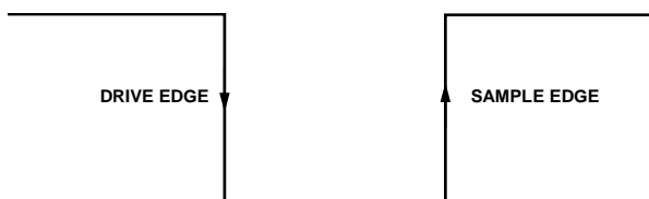
Figure 25. SPI Mode 3 SCLK Edges
