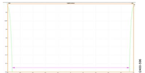
Figure 134. Bathtub, External 100Ω Terminations at 6 Gbps
