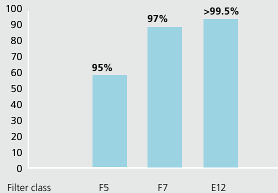
Medium filtration efficiency Em % against particle size 0.12 \mu\text{m}
