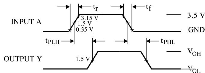
Figure 1. Switching Waveforms
