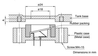
The transducer can beak off if the A dimension depth is shallow. TDK recommends a 2mm A-dimension depth and a screw tightening torque of  $0.6N \cdot m$ .
