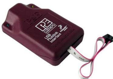
**Figure 9-1: P&E's USB Multilink (USB-ML-12 shown)**
