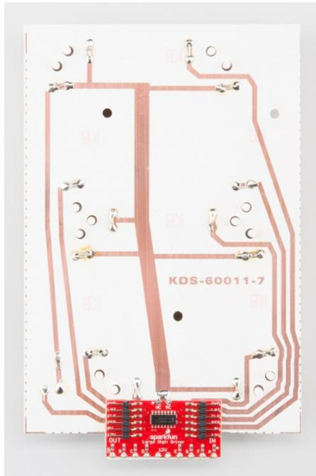
Several Large Digit Drivers can be chained together to create a display with multiple digits.
