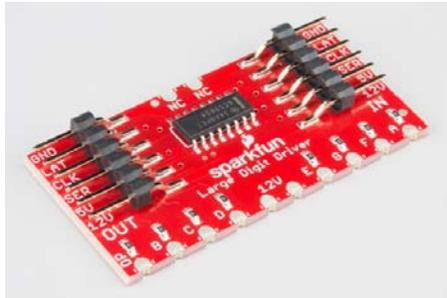
The Large Digit Driver can be soldered directly to the bottom of the 7-Segment Display.
