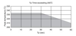
• Above "Reflow Profile" graph indicates temperature at the terminals and capacitor top.
