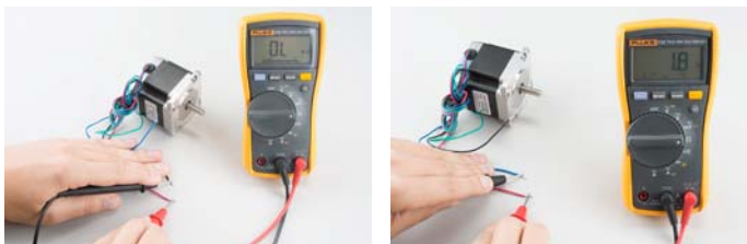
Here you can see that the first two random wires measured open, and the second two measured 1.8 ohms. This is a typical large-ish 2 phase stepper.
