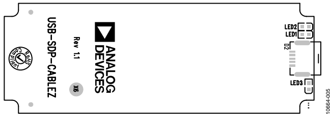
Figure 5. USB-SDP-CABLEZ Board LEDs
